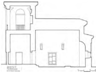
Fig. 2. Church of St. Demetrius in Veles. Longitudinal section according to S. Korunovski
